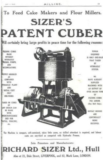
This year sees Sizer Limited celebrate the centenary of its innovative Cuber patent. Sizer's 'Patent Cuber', developed in 1911, was designed for feed cake makers and flour millers. The revolutionary design meant that industry no longer needed to run large, expensive, hydraulic presses and pumps – the traditional production method at the time.
