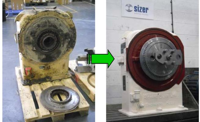
Service Engineer, Graham Turner, explains the process, "Usually our customers will ask us to assess their current machine, and we are able to detail the replacement parts required and lead times. The press is then sent to our factory in Rotherham, South Yorkshire, for complete refurbishment, alignment, bearing and seal changes, painting and running in." He continues, "We then can re-install the press and commission it so that our customers have as little down time as possible."
